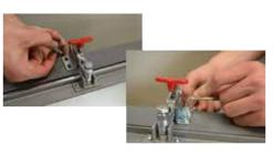
**Step 2** Using the four (4) bolts and nuts provided, attach the material hold down bracket to the table.
